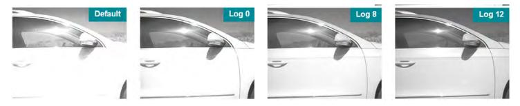
The sensor allows capturing highly dynamic scenes at best image quality even in difficult light conditions and global shutter mode thanks to its Log-mode feature. Log-mode parameters can easily be adjusted via uEye Cockpit to get the best setting according to the requirements of various situations. Hence, the sensor is the perfect replacement for costly HDR sensor solutions.
